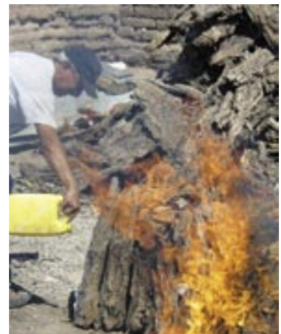
After stacking two layers of wood around the planter, Andreas pours kerosene on it and ignites it. It will need to burn until all the wood has turned to ash in order to completely fire the vessels.
